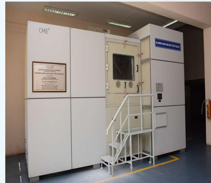
**Blowing Sand & Dust Test Facility**
