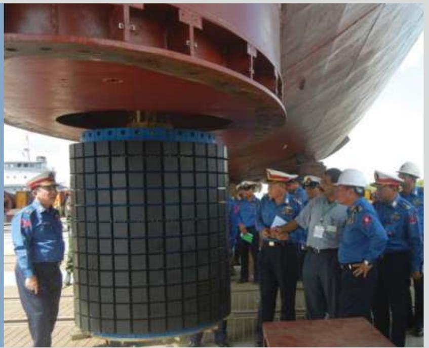
**HMS-X ARRAY ONBOARD A DESTROYER CLASS SHIP**
