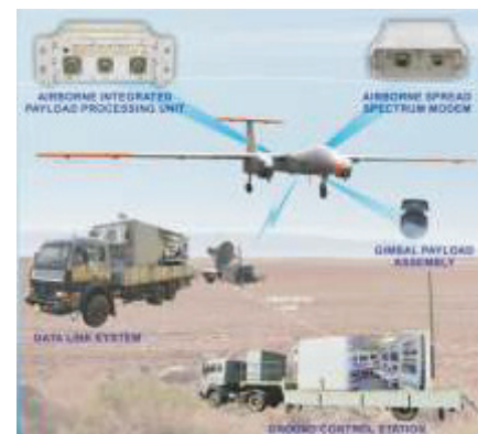
GCS & Datalink Deployment for Rustom UAV
